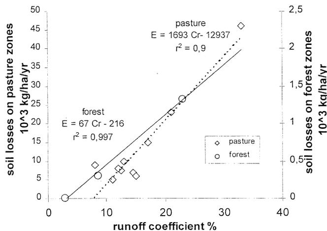
Fig. 2. Relationship between measured soil losses ( $E$ ) and calculated runoff coefficient ( $Cr$ ) on plots of 50 m<sup>2</sup> located on pasture (p) and forest (f) zones. Straight lines correspond to fitted linear regression.  $r^2$  = Coefficient of determination.
