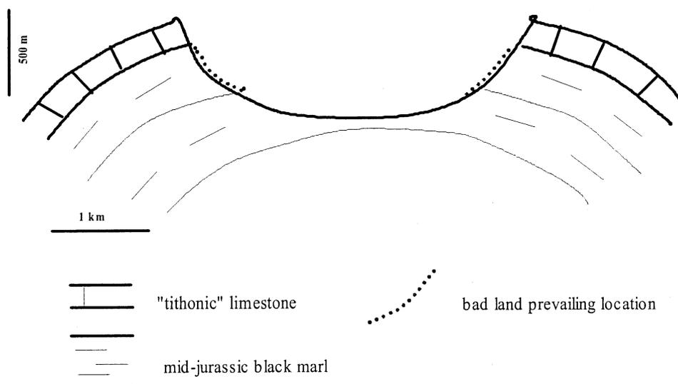
**Fig. 3** The prevailing location of badlands on a cross section of a typical valley of the “Vocontian Graben” badlands are mostly located where the slope gradient and the intensity of overland flow are high. This explains why the dip–hillslope angle is commonly between 60 and 90°.
