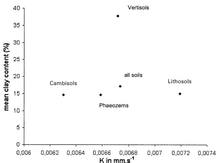
Fig. 3. Clay content vs  $K$  ( $-10$  mm) for the different soil types.
