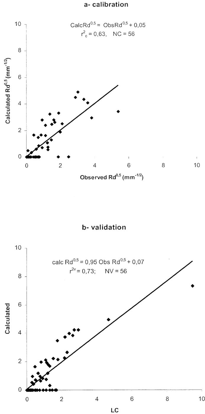
Fig. 6. Calibration (a) and validation (b) of NAZASM for the plot 22 (area = 50 m<sup>2</sup>; El Aguaje site, 1996–1998): comparison between calculated and observed values of runoff (square root).
