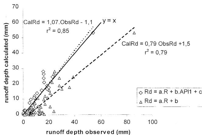
Fig. 3. Comparison between calculated (CalRd) and observed (ObsRd) runoff depth, for plot 22 (1996 and 1997), using the regression  $Lr = aR + b\text{API} + c$  and a simple regression  $Lr = aR + b$ .  $R$  = Rainfall amount (mm).  $r^2$  = Coefficient of determination.
