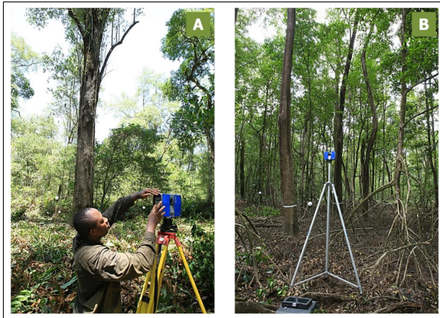
Figure 1-4: Setting up the FARO 3D X330 laser scanner on a tripod in the mangrove forests
