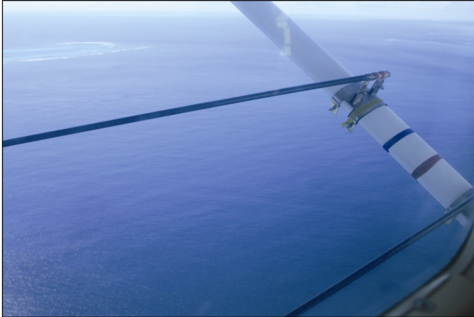
Figure 2.3: Fiberglass rods attached to the structure of the aircraft to delineate transects 400m wide on the water surface on each side of the aircraft. Note the colour bands on the wing strut that were used to delineate zones within the transect.
