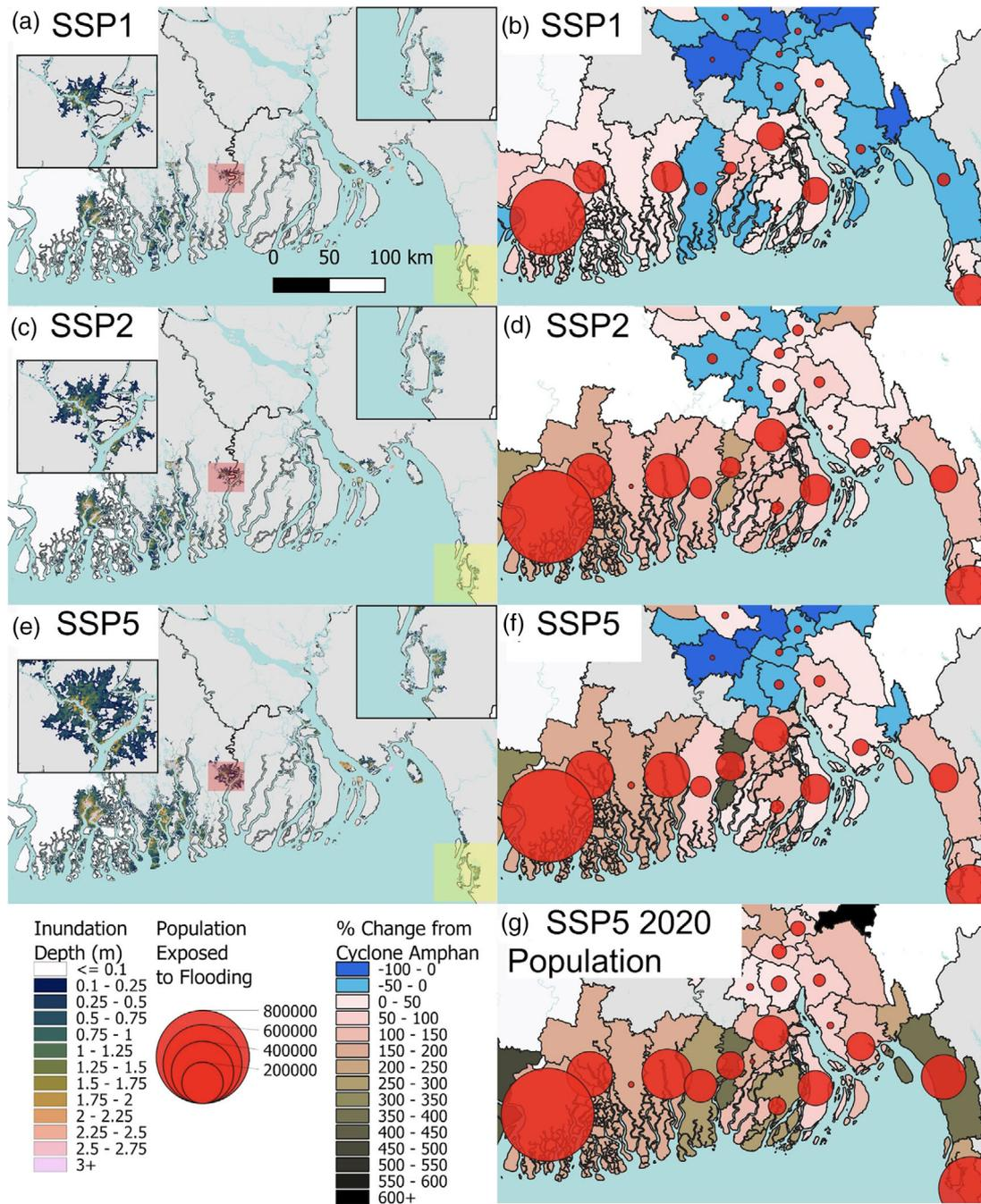
**FIGURE 5** Projections of the flood inundation and exposure for Super Cyclone Amphan under different climate scenarios. Panels (a–f) are as in Figure 3, but for the three different sea level rise scenarios predicted for 2100. The blue and green colours now show the percentage change in exposure from the 2020 baseline. Panel (g) shows the same as panel (f), but keeping the population at 2020 levels
