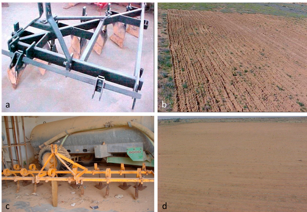
Figure 2. Ploughing tools used during the field experiment: (a) the moldboard plough, and (c) the tiller plough and photographs of the corresponding parcels after tillage operations ((b) and (d), respectively).
