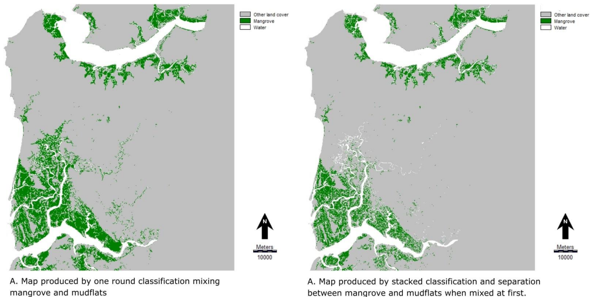
Figure 6. Comparison of mangrove map of 1986 LANDSAT imagery between one round ISODATA classification (A) and Stacked classification in order to subdivide mixed classes (B).
