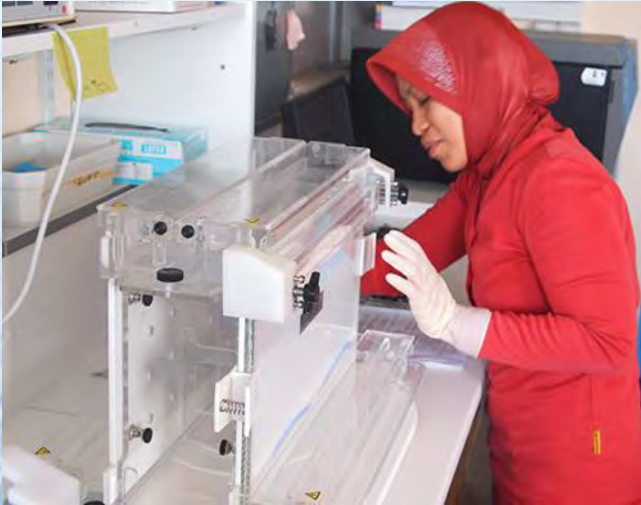
Irma S. Arlyza preparing a vertical polyacrylamide gel at P. Berrebi's laboratory in Montpellier
