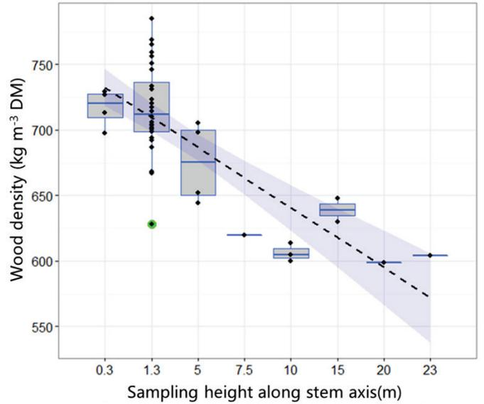
**Fig. 3** Decreasing wood density at different heights along the stem axis: black dots denote the wood density values obtained from various tree samples; the green dot was consider an outlier; and the dashed line shows the linear model with a 95% confidence interval in blue
