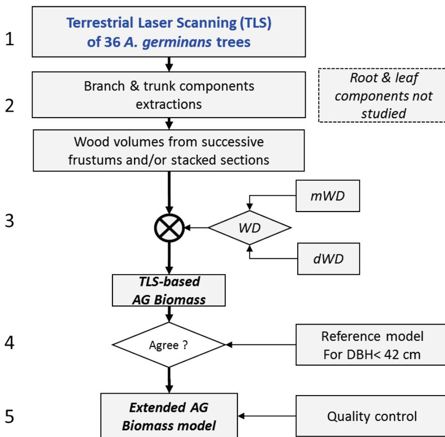
**Fig. 1** Scheme of procedure for TLS data acquisition and processing in mangrove tree biomass estimation. AG = aboveground, *WD* = wood density, *mWD* = mean *WD* value at tree *DBH*, and *dWD* = decreasing value of *WD* with height along the stem axis
