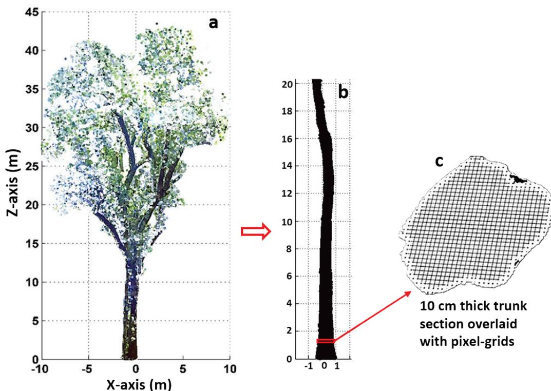
**Fig. 2** Trunk segmentation and sectioning for stem volume computation. a) Typical view of a large mangrove tree. b) A trunk with  $DBH = 93.5$  cm. c) Typical flattened projection of a trunk section extracted at a height of 1.3 m
