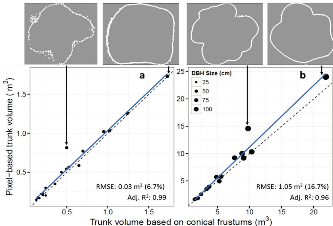
**Fig. 4** Comparison of the trunk volumes estimated using the automatic pixel-based analysis of TLS data and the successive trunk-fitted conical frustums for trees with *DBH* < 42 cm (a) and > 42 cm (b). Outline of girth form of typical trunks are shown above in white with a grey background (arrows 1–4). The dashed line depicts a one-to-one relationship and the blue solid line corresponds to linear fit.
