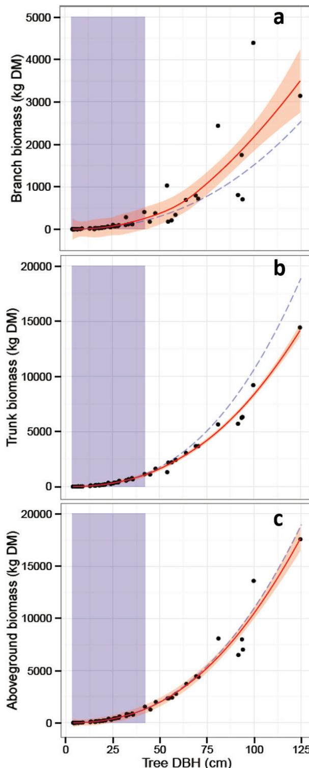
**Fig. 6** Comparison of the TLS-based biomass functions and the reference models for *A. germinans*. The branch (a), trunk (b), and total AGB (c) are distinguished. The red line and the surrounding shade represent the new model and confidence interval. The dashed line is the prediction from the reference model, calibrated over the *DBH* range in the shaded area
