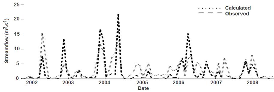
Fig. 7: Calculated and Observed streamflow at Abadla Station
