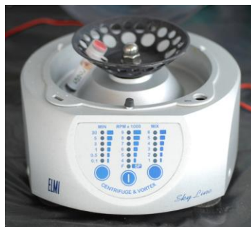
Figure 18: Example of microcentrifuge suitable to realize serum in a field laboratory (Photo: Herbreteau V.)
