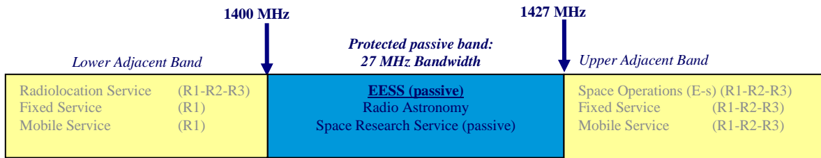
Figure 3: Schematic about frequency allocation to the EESS passive in the 1400-1427 MHz band
