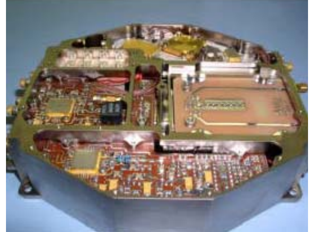
Fig. 2b. LICEF: individual receiver element of MIRAS. © Mier Comunicaciones
