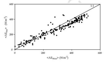
**Fig. 9.** Comparison between the estimated ( $\langle AE_{Sim} \rangle$ , obtained using the temporal aggregation scheme (Eq. (22))) and observed ( $\langle AE_{Meas} \rangle$ , obtained as area-weighted averages of those measured over both sites) area-averaged available energy.
