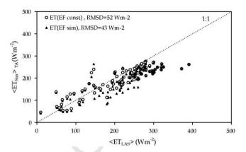
**Fig. 10.** Comparison between  $(ET_{Sim})_{TA}$  (estimated using the temporal aggregation scheme through Eqs. (19)–(23)) and  $(ET_{LAS})$  (obtained form the LAS as the difference between the  $(AE_{Meas})$  and  $(H_{LAS})$ ). Also included is the **grid-scale** evapotranspiration calculated by considering a constant diurnal evaporative fraction (EF) equal to that at 11:30 UTC (EF<sub>1130</sub>).
