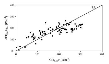
Fig. 12. Comparison between  $(ET_{Sim})_{TA}$  (estimated using the temporal aggregation scheme (Chehbouni et al., 2008a)) and  $(ET_{LAS})$  (obtained form the LAS, Chehbouni et al., in press).
