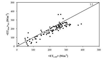
**Fig. 8.** Comparison between  $\langle ET_{Sim} \rangle_{SA}$  (estimated using the spatial aggregation scheme) and  $\langle ET_{LAS} \rangle$  (obtained form the LAS as the difference between the  $\langle AE_{Meas} \rangle$  and  $\langle H_{LAS} \rangle$ ).
