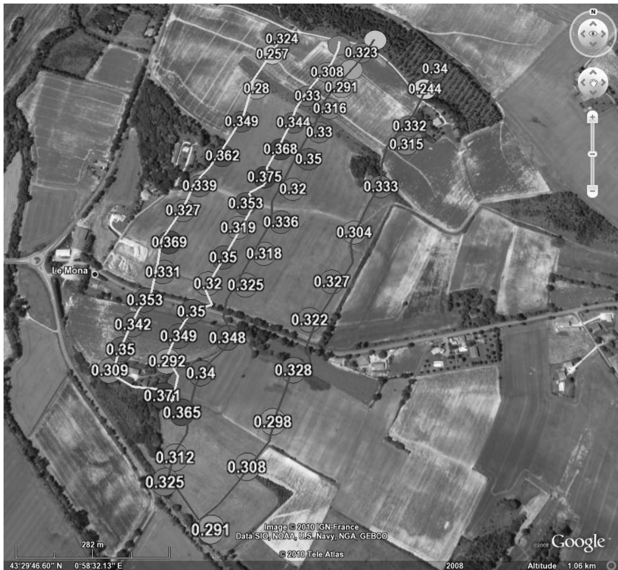
Figure 4 : Illustration of soil moisture acquisition on the Le Mona site for 2010 April 28. Soil moisture is measured with ThetaProbes by two teams (yellow and red line).
