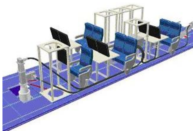
Figure 2. The CAROLS radiometer inside the ATR42 research aircraft, (a) illustration of nadir antenna inside the aircraft, (b) illustration of CAROLS system (receiver and antennas) inside the aircraft.
