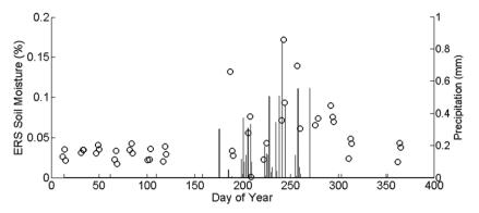
Fig. 5. Comparison between precipitation measurements (bars) in Kafina (13.71°N 2.73°W) and estimated soil moisture content (mm) using ERS remote sensing products (circles).
