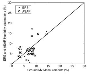
**Fig. 4.** Inter-comparison between ground data and ERS ( $\times$ ) and ASAR ( $\bigcirc$ ) surface soil moisture products for the Niger.
