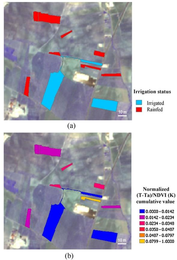
**Fig. 12.** (a) Irrigated (blue) and rainfed (red) orchards over the study area acquired on 21 September 2005 with ASTER sensor; (b) normalized cumulative  $(T - T_a)/NDVI$  value calculated for each field over the entire study period.
