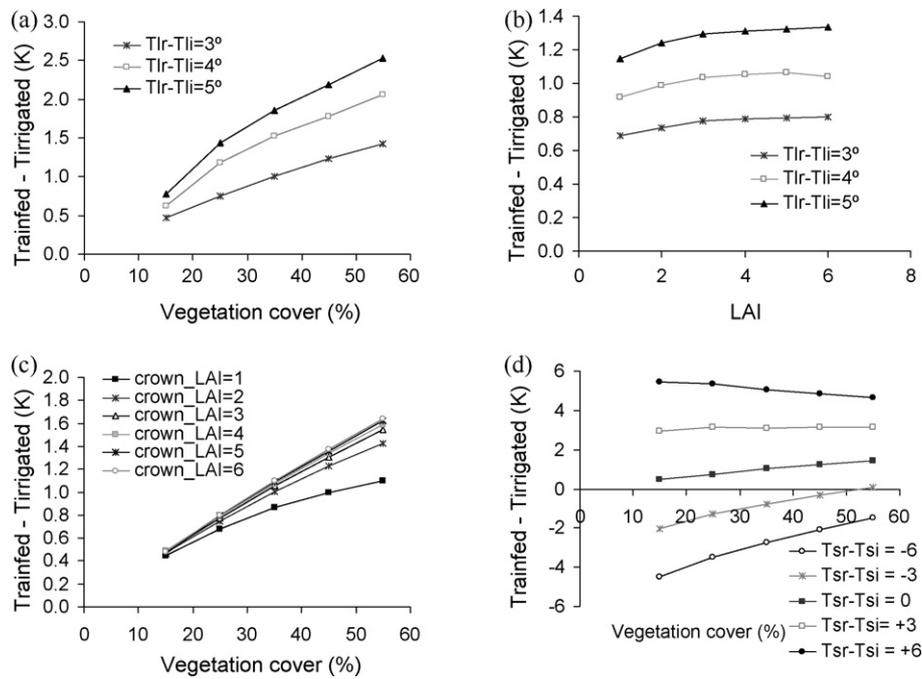
**Fig. 13.** DART simulations obtained for rainfed minus irrigated orchard temperature as function of percentage cover for different  $T_{rainfed} - T_{irrigated}$  leaf gradients ( $T_{lr} - T_{li}$ ) (a); effects of crown LAI for different  $T_{rainfed} - T_{irrigated}$  leaf gradients (b), effects of percentage cover for different crown LAIs (c), and effects of percentage cover for different  $T_{rainfed} - T_{irrigated}$  soil gradients ( $T_{sr} - T_{si}$ ) (d).
