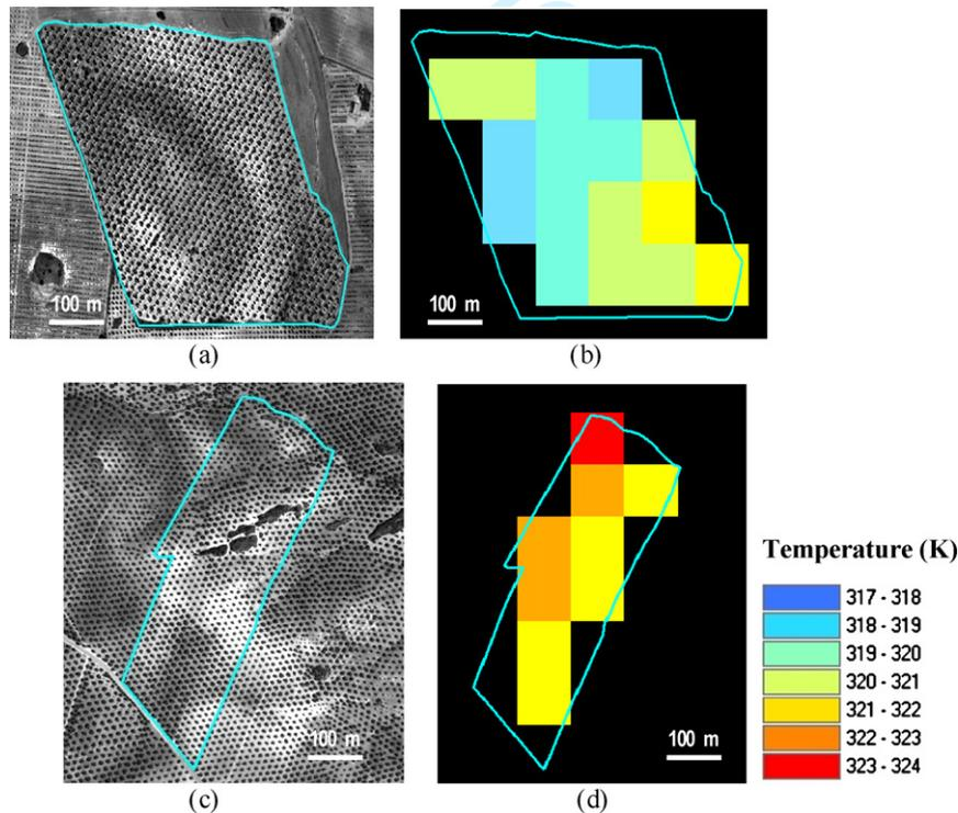
**Fig. 10.** Orthophotos acquired for an irrigated olive orchard (a) and a rainfed orchard (c) with same vegetation percentage cover (25%) and same NDVI (0.18), showing their corresponding ASTER temperature images (b and d).
