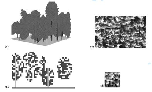
Fig. 6. Fir forest plot in the Tancítaro site: simulated 3D structure (a) and vertical 2D profile at 1 m resolution (b). Panchromatic IKONOS (c) and DART (d) images of the forest plot. The DART panchromatic image is derived from a fusion of DART multi-spectral images.
