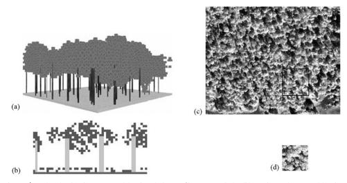
Fig. 5. Pine forest plot in the Tancítaro site: simulated 3D structure (a) and vertical 2D profile at 1 m resolution (b). Panchromatic IKONOS (c) and DART (d) images of the forest plot. The DART panchromatic image is derived from a fusion of DART multi-spectral images.
