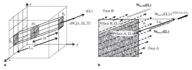
Fig. 6. Computation of the TIR emission of a turbid cell  $(T, u_f, LAD)$
