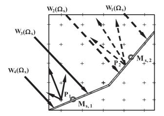
**Fig. 4.** Interception of 4 rays by 2 figures.  $W_1$  and  $W_2$  are intercepted by Fig. 2.  $W_3$  and  $W_4$  are intercepted by Fig. 1. Resulting effective points of emission are  $P_2$  and  $P_1$
