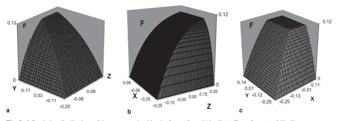
**Fig. 8.** 3-D relative distributions of the energy emitted by the faces of a turbid cell. (a) Front face  $(x = \Delta X)$ : F(y, z, LAI, LAD). (b) Right face  $(y = \Delta Y)$ : F(x, z, LAI, LAD). (c) Top face  $(z = \Delta Z)$ : F(x, y, LAI, LAD). LAI = 5.  $\Delta Y = \Delta Z = 0.5$ . LAD spherical.  $(\theta_v, \theta_v) = (60,72)$
