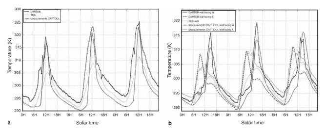
**Fig. 15.** Comparison of temperature measurements with DARTEB and TEB simulations. July 14–16 2004. (**a**) Road of La Pomme street (Toulouse) with a south East – North West orientation. (**b**) Walls of Alsace Lorraine street (Toulouse) with a South-North orientation. The 2 walls are facing West and East directions, which implies different thermal behaviors
