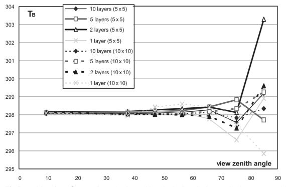
Fig. 7. Precision of  $T_{app}(\Omega_v)$  according to the view zenith angle, the discretization  $N_{sf}$  (5 × 5 or 10 × 10) and the numbers of layers (1–10). LAI=5.  $T_f = 298$  K
