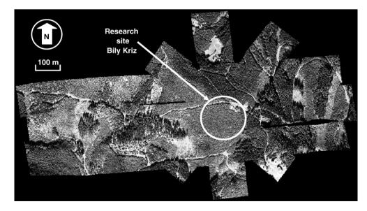
Fig. 5. Six ortho-rectified flight lines acquired by the airborne AISA Eagle imaging spectroradiometer in a multi-directional pattern with the pixel size of 0.4 m over the permanent experimental research site Bily Kriz (Beskydy Mts., Czech Republic; 18.54 °E, 49.50 °N, altitude 936 m above sea level; greyscale image of NIR, red, and green band composition).
