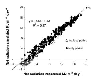
Fig. 1. Simulated vs. measured daily net radiation (MJ m<sup>-2</sup>) during 1997. Results are separated between leafy period ( $\bullet$ ) and leafless period ( $\Delta$ ).
