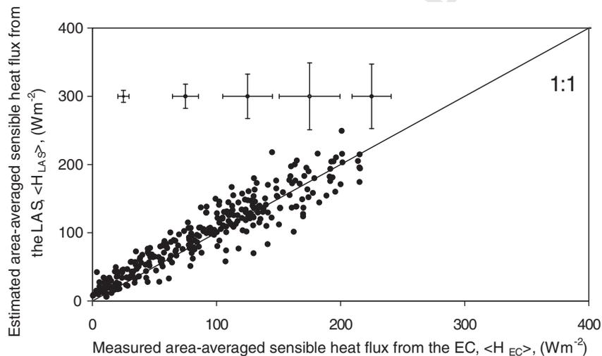
Fig. 4. Comparison between measured—derived from the EC systems,  $\langle H_{EC} \rangle$ —and estimated—derived from the LAS,  $\langle H_{LAS} \rangle$ —area-averaged sensible heat fluxes during the study period (DOYs 204–225). The error bars represent the average uncertainty of the fluxes for each 50  $\text{W m}^{-2}$  interval.
