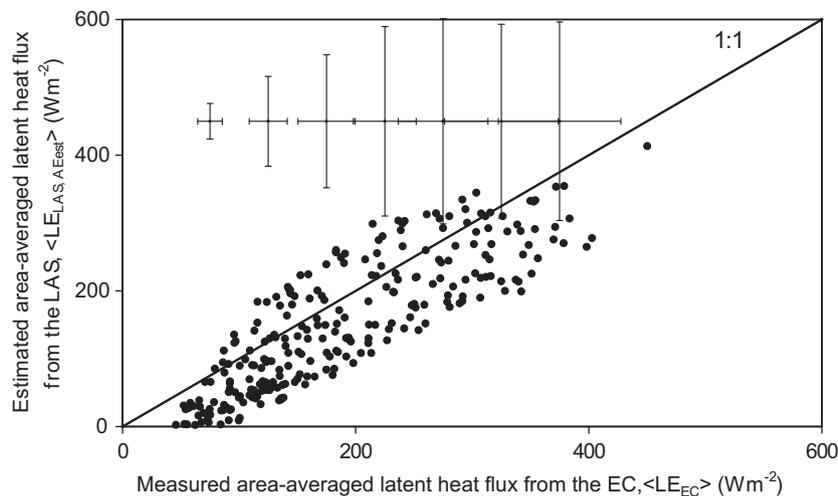
**Fig. 7.** Comparison between measured—derived from the EC systems, ( $\langle LE_{EC} \rangle$ )—and estimated—derived from the LAS using the estimated available energy, ( $\langle LE_{LAS, AE_{est}} \rangle$ )—area-averaged latent heat fluxes during the study period (DOYs 204–225). The error bars represent the average uncertainty of the fluxes for each  $50 \text{ W m}^{-2}$  interval.
