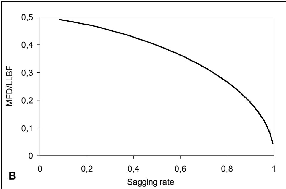
**Figure 2.** Theoretical relationship between the ratio MFD/LLBF and the angle ( $0^\circ < \varphi < 90^\circ$ ), (panel A) and SR ( $0 < SR < 1$ ), (panel B). MFD is the theoretical maximum depth, LLBF is the length of the mainline between floats and SR is the sagging rate. On this figures the value of the length of floatline (LF) and the length of branchline (LB) is supposed equal to zero.
