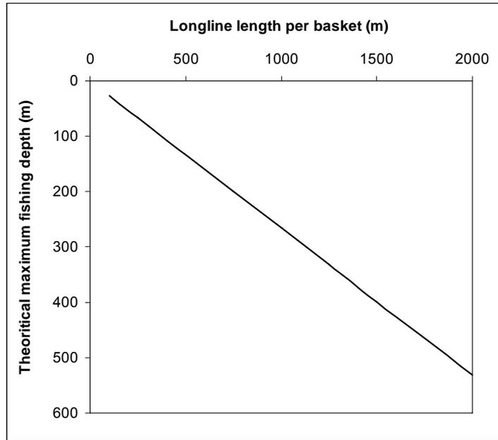
**Figure 4.** Relationship between the theoretical maximum fishing depth and the length of the longline between floats for a sagging rate of 0.8 ( $\varphi = 56^\circ$ ) according to a catenary geometry.
