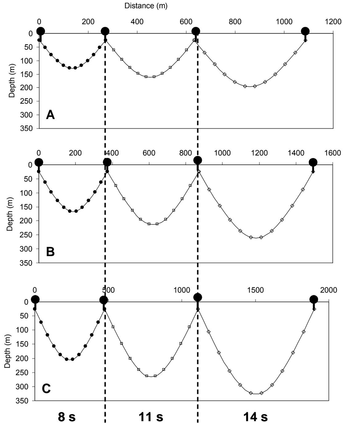
**Figure 3.** Variations of the theoretical maximum fishing depth of the mainline for similar baskets (10 hooks, sagging rate = 0.76) according to different time intervals between hooks (8 s, 11 s, 14 s) and setting speeds of boat (A = 6 knts, B = 8 knts, C = 10 knts).
