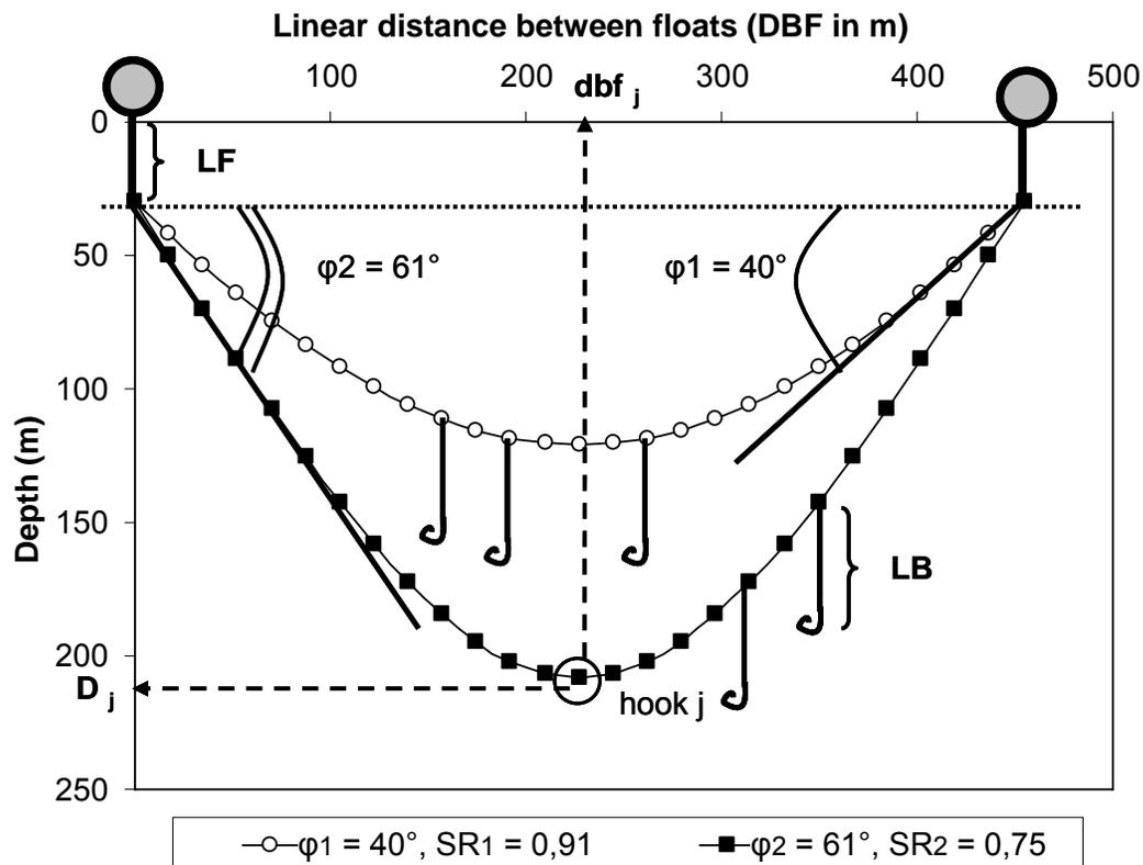
**Figure 1.** Theoretical catenary shape of two baskets defined by respective values of the sagging rate of 0,91 ( $\phi_1 = 40^\circ$ ) and 0,75 ( $\phi_2 = 61^\circ$ ).  $D_j$  is the depth of the hook  $j$  located at a distance  $dbf_j$  form the floatline, LF is the length of the floatline and LB is the length of the branchline (see text for the corresponding catenary equation).
