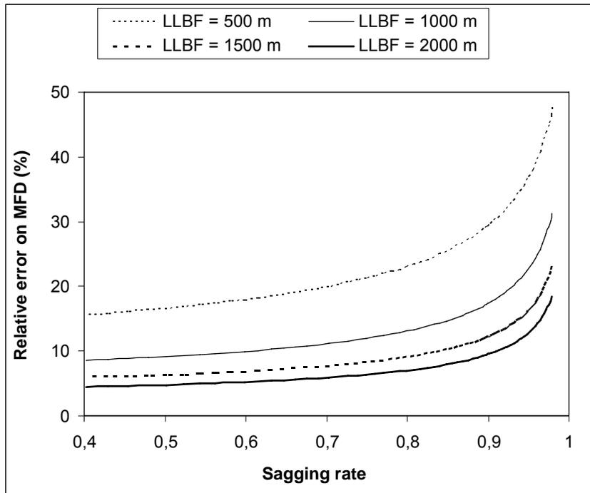
**Figure 6.** Relationship between the relative error on the theoretical MDF (%) and the sagging rate according to different lengths of the mainline per basket if the length of the floatline (LF = 40 m for this example) is unknown.
